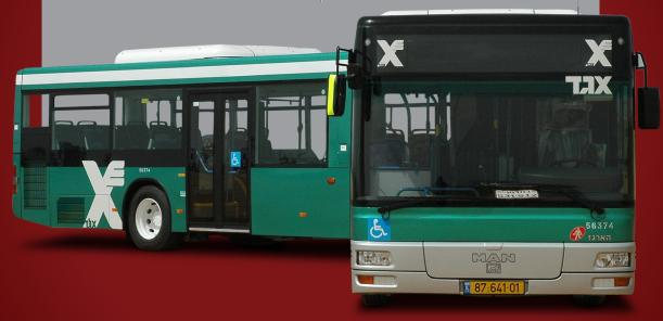
The main difference is the advanced state-of-the-art defense which is not readily apparent since the look of the Barak 21 is preserved in appearance, design, safety & quality. The stringent international overturning standard R-66 complying bus protects against gun-shots & has an armored windshield which is divided into two parts, providing increased protection for the passengers.
