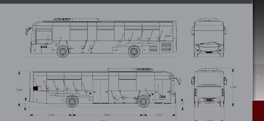
Chassis MAN A69 Overall length 12300 mm Overall width 2550 mm Total height 3205 mm Internal height 2550 mm Wheelbase 5980 mm Gross vehicle weight 18000 kg Seating capacity 38+1 Standing capacity 52 AC unit 35 kw Engine MAN D0836 LOH60 Max torque Gear box Tires Air bellows Brake units Fuel tank
