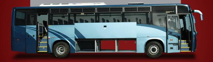
The R-66 European standard compliant bus structure is passivated against corrosion, taking into consideration phosphate treatment & painting with protective epoxy paint.
